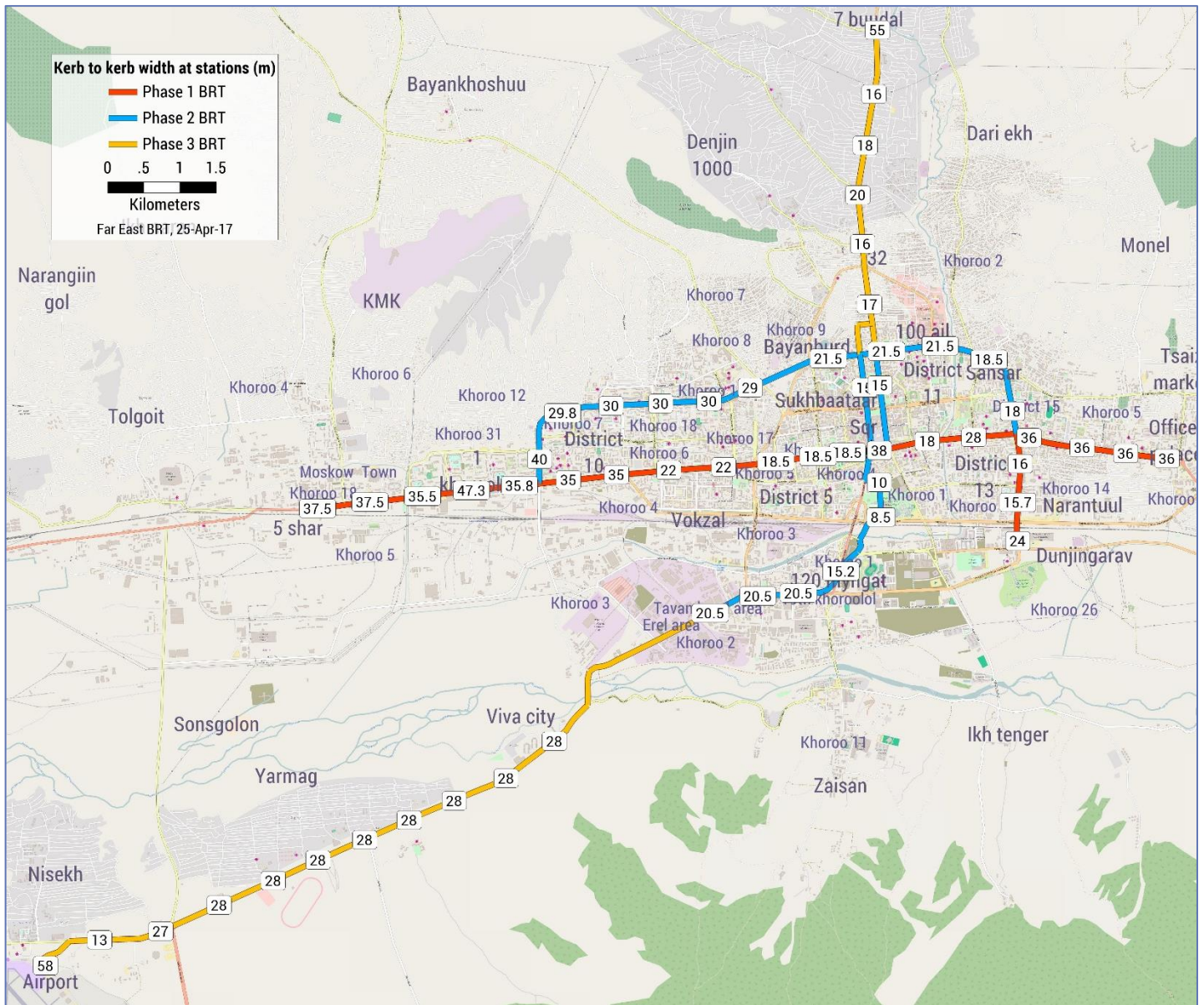
Kerb to kerb width at BRT stations.
