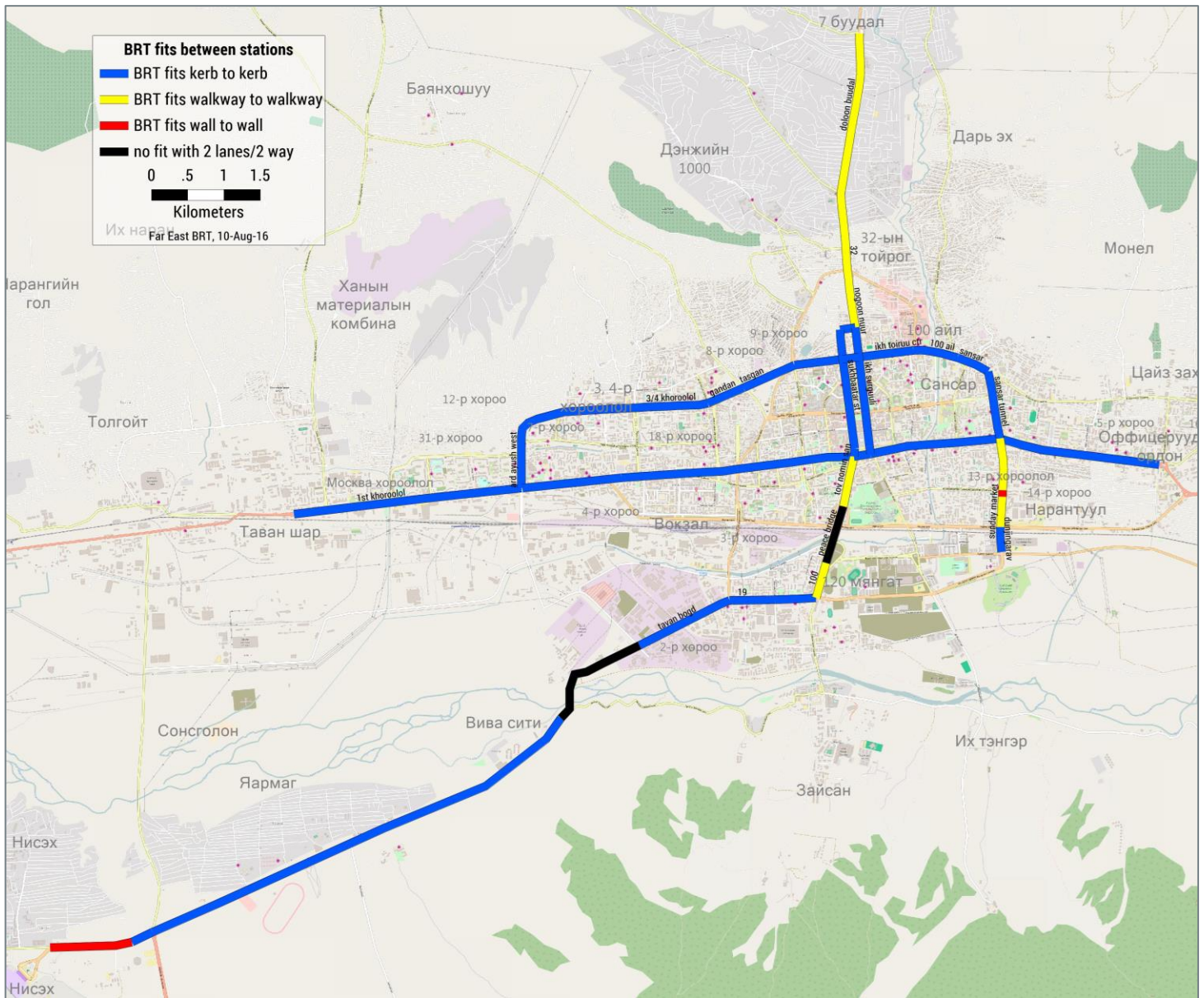
BRT fits between stations. A modified alignment was developed to avoid Peace Bridge.
