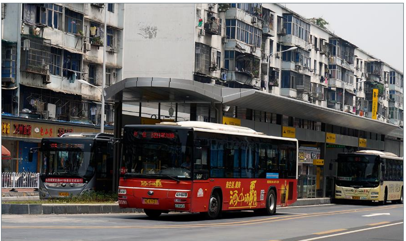
In the directional BRT stations in the main BRT corridor in Yichang, a mix of pre-existing and new BRT buses are used. The stations accommodate buses with doors in the right side only, and with doors in both sides.
