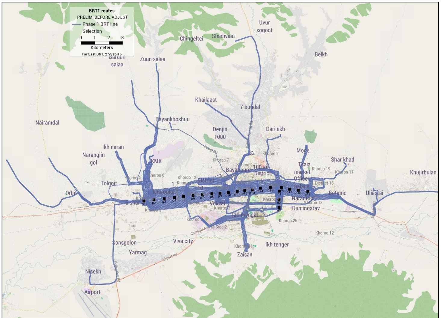
Expanded route selection of 32 phase 1 BRT routes – before adjustment. The route selection needs to be done as part of the preliminary operational design which ideally involves developing a BRT model with the smart card data as the basis and starting point.
