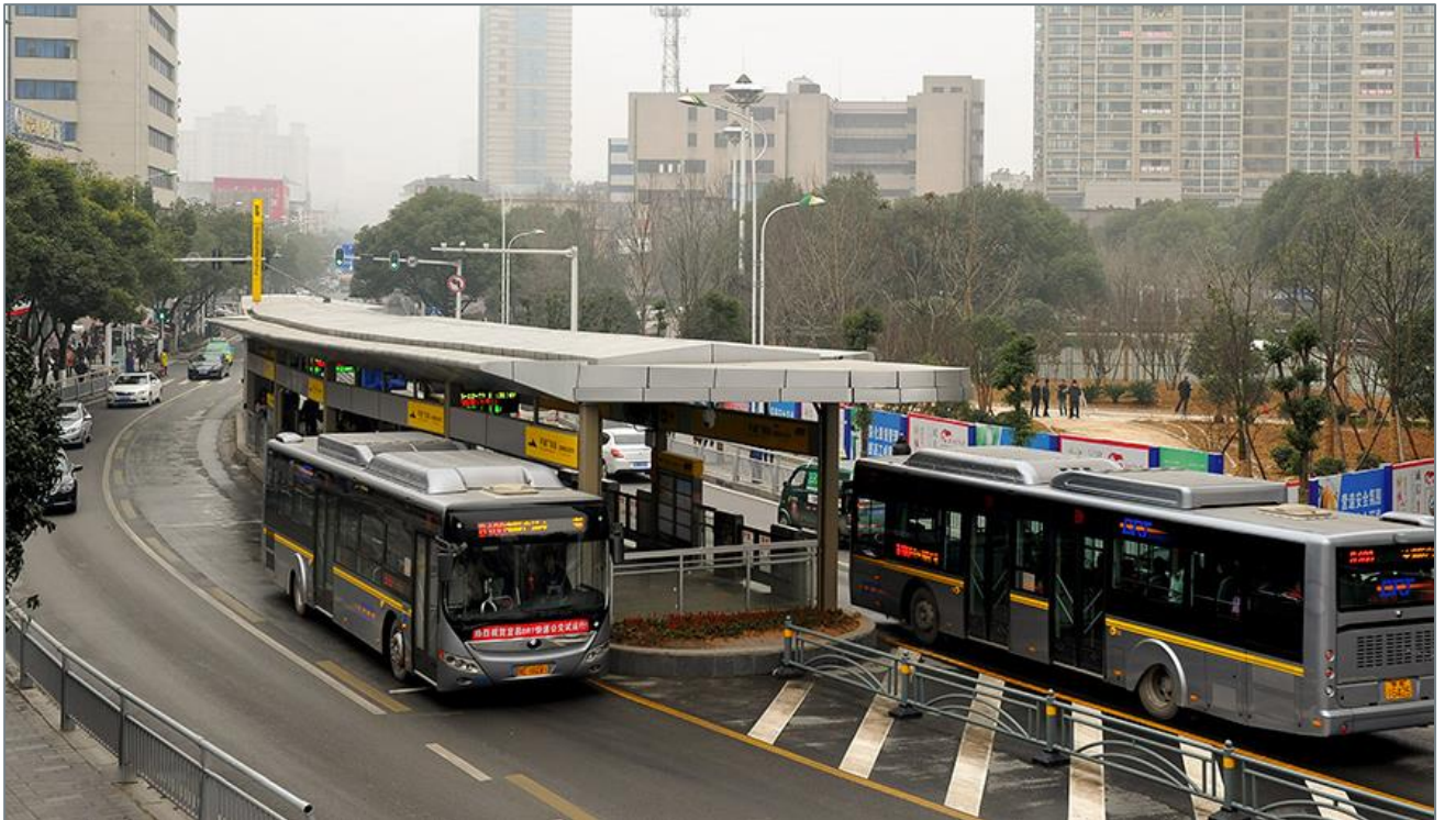
12m BRT buses with two doors in both sides in Yichang, in the northern part of the corridor where stations do not have overtaking lanes. Ulaanbaatar will have BRT buses with similar dimensions.
